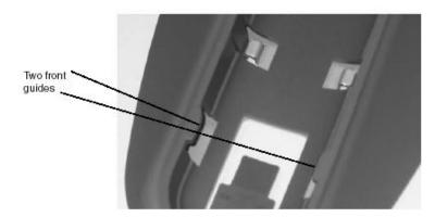
Slide the base in from the rear of the unit, by using the locating guides.
