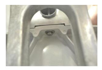
Underside view of screw through arm, main arm and dish.
