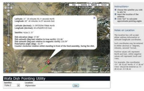
This will display the azimuth and elevation to set on your dish to start looking for the satellite.
