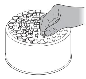
Loading the syringe and needle rack
